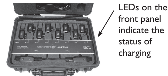
Figure 2: Plugging Charging Cable Jacks into Microphone/Transmitters and Pendant Receivers
